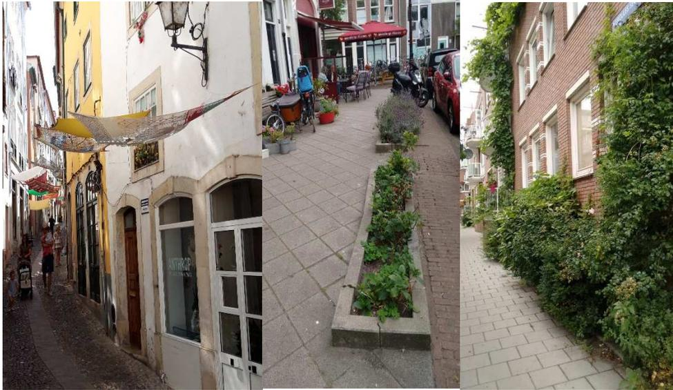
**Figure 5** implemented measures to tackle climate change effect such as heat stress. Left: shading provided by cloth over shopping streets in Coimbra, Portugal. Right: stones removed from urban dense area of Amsterdam for lower temperatures and infiltration of stormwater (source: [www.climatescan.nl](http://www.climatescan.nl))
